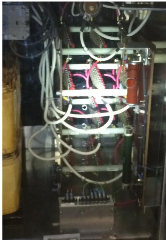
The picture above shows the high voltage rectifier stack, high voltage filter, and spark gap.
