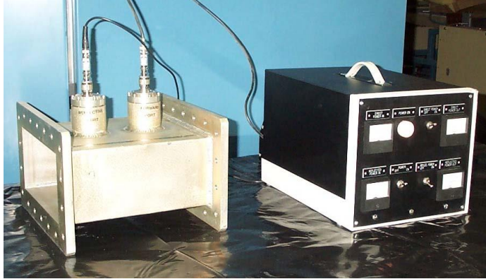
The above picture shows a Portable Microwave Power Meter.
