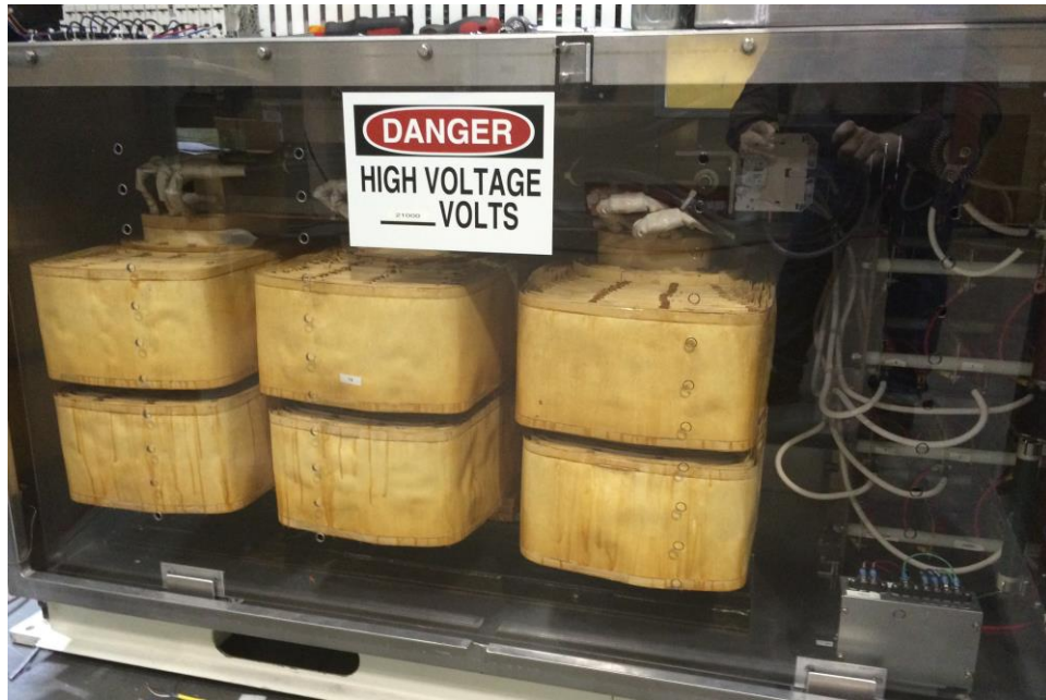
The above picture shows the High Voltage Power Supply section (with the protective cover removed). The anode transformer and rectifier assembly are visible on the front plane.
