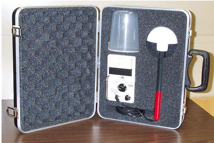
The above picture shows a Microwave Oven Survey Meter – Model HI-1600 and its carrying case.
