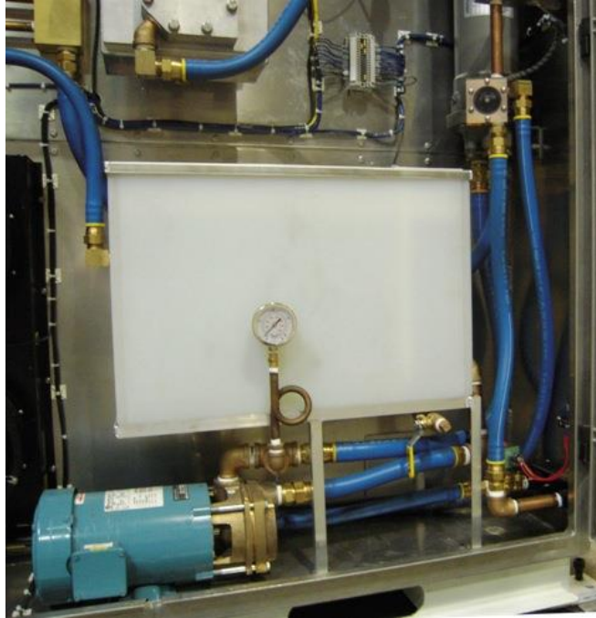
Above is the distilled water tank, water pump, and cooling water inlet and outlet connections.
