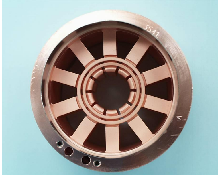
Shown above is the anode of the magnetron with its resonant cavities.
