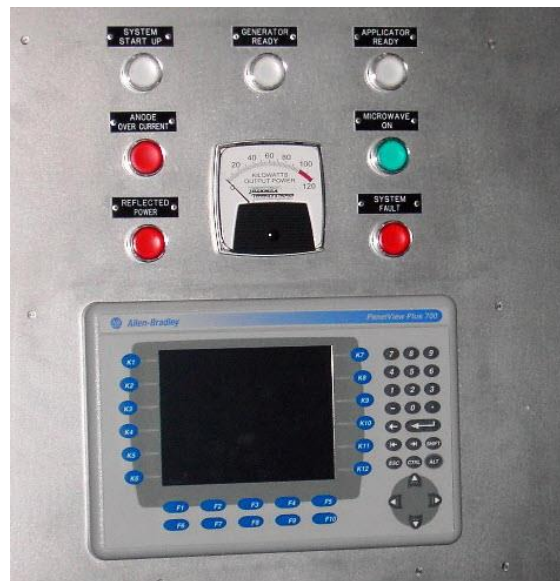
A closer look at the Generator Control Panel with the PanelView Operator interface is shown above.
