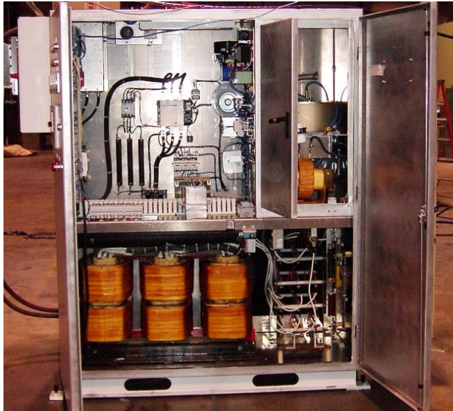
Front view of the MW generator cabinet.
