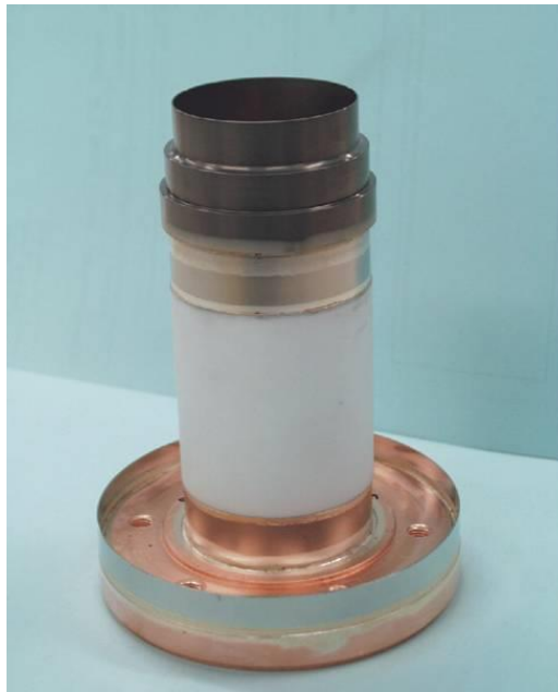
Ceramic insulation with metal seals.
